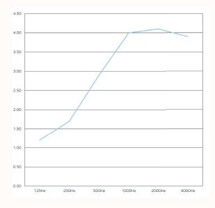
The graph represents the equivalent absorption surface area for an object (Aeq). Measurement used Pink Noise as excitation signal in a reverberant room.
