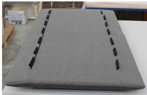
Once the tab is pushed through this gap, a rubber cylinder is pushed into the tab to secure it.
