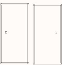
Panel: 900mmW Switch Height: 960mm Depth from Left/Right Side: 100mm Switch panel opposite shelf panel
