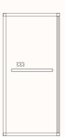
Shelf Panel with Power OutletPanel:900mmWPower Outlet Height:1130mm
